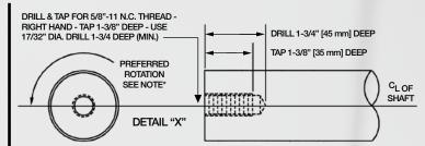
\*NOTE: When threaded stub shaft (Part 303 or equal) is to be used. It is recommended that the location of the stub be in the end of the shaft that rotates counterclockwise. This allows the threads to continue being under a constant fastening torque while the shaft turns. If the rotation is clockwise or the shaft is for reversing type service, make sure the jam nut is locked tight against the shaft.
