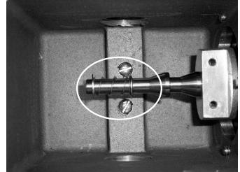
Figure 10: Switch assembly, spring retainer, spring with washers and machine screws with washers.
