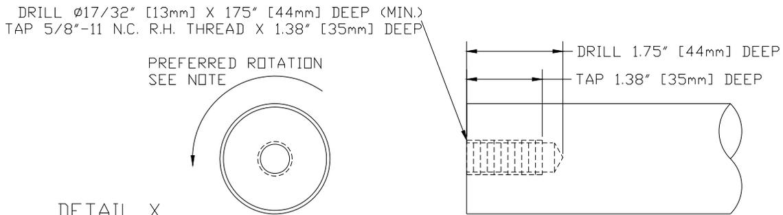
NOTE: WHEN THREADED STUB SHAFT (PART NO. 303) IS USED, IT IS RECOMMENDED THAT THE LOCATION OF THE STUB BE IN THE END OF THE SHAFT THAT ROTATES COUNTER-CLOCKWISE. THIS ALLOWS THE THREADS TO CONTINUE BEING UNDER A CONSTANT FASTENING TORQUE WHILE THE SHAFT TURNS. IF THE ROTATION IS CLOCKWISE OR THE SHAFT IS FOR REVERSING TYPE SERVICE, MAKE SURE THE JAM NUT IS LOCKED TIGHT AGAINST THE SHAFT.
