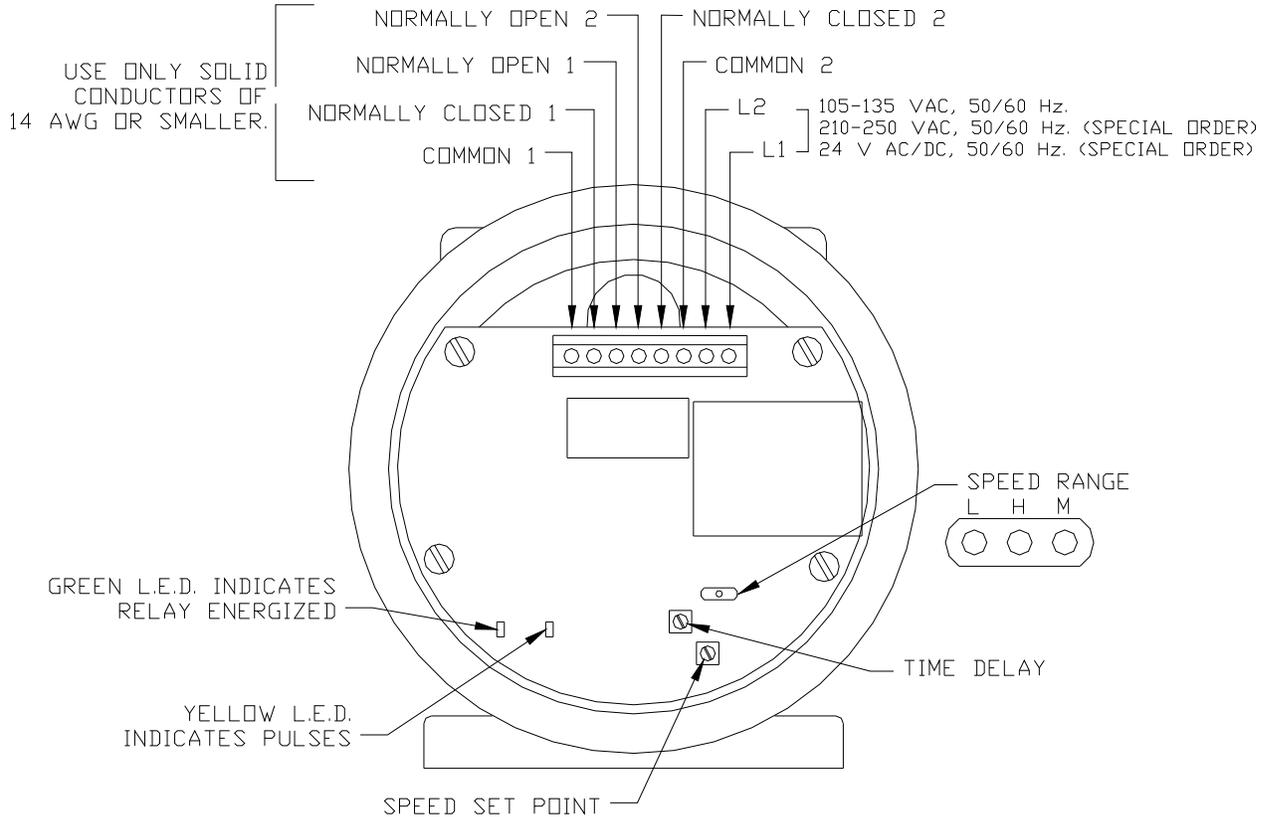
Remove end cap to expose terminals and pick-up speed adjustment screw. Wire input power from source to terminals L1 & L2. Be certain to use the provided ground screw. The output of the model CMS is a DP/DT relay. There are two sets of output contacts. Each set includes normally open, normally closed and common. As a result, the unit can be used to control two separate circuits such as a motor starter and a signal light.
