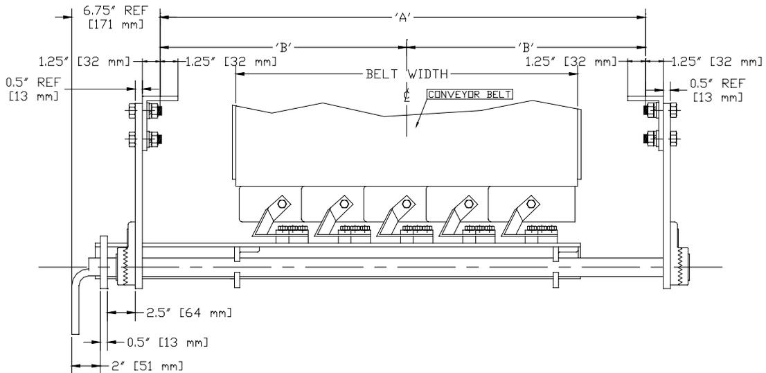
Figure 2: Hanger Rail Mount Side View
