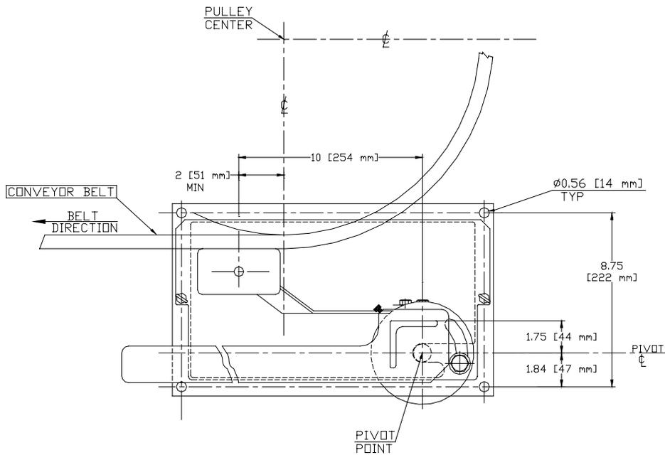
**Figure 5: Chute Mounting Dimensions**
