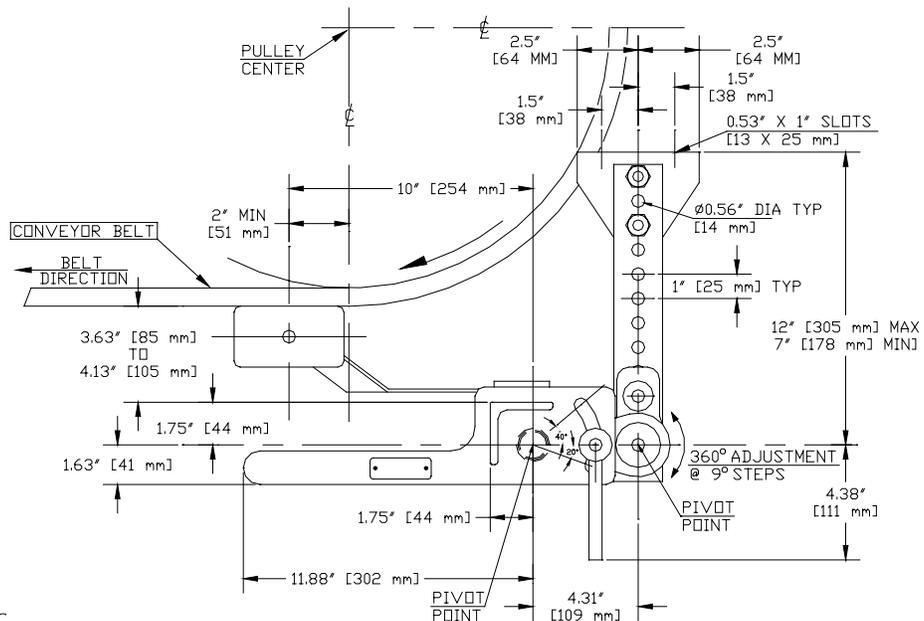
**Figure 3: Chute Mount Unit Dimensions**
