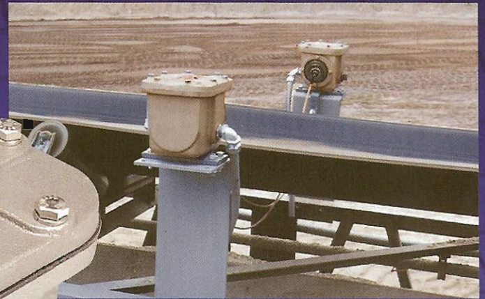
VIEW OF CONVEYOR SHOWING UNIT MOUNTED WITH CABLE UNDERNEATH (2 REQUIRED)
